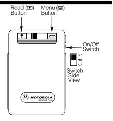
**READ Button:** (**ID**) - Used to read messages and to activate pager functions. Also used to scroll through the hours and minutes digits for time setting.
