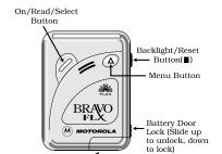
Slide battery door to the right (Insert positive end of battery first) ACPB-952422-0
