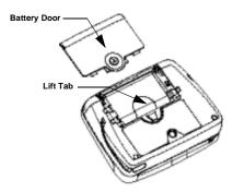
3. Using the white lift tab, lift the battery from the battery compartment.
