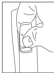
a. Pry dust cover from body.
