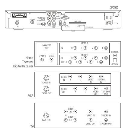
Use this diagram to record cable connections on the rear panel. Later, you can use this diagram to reconnect your system if you move the equipment or add new equipment.
