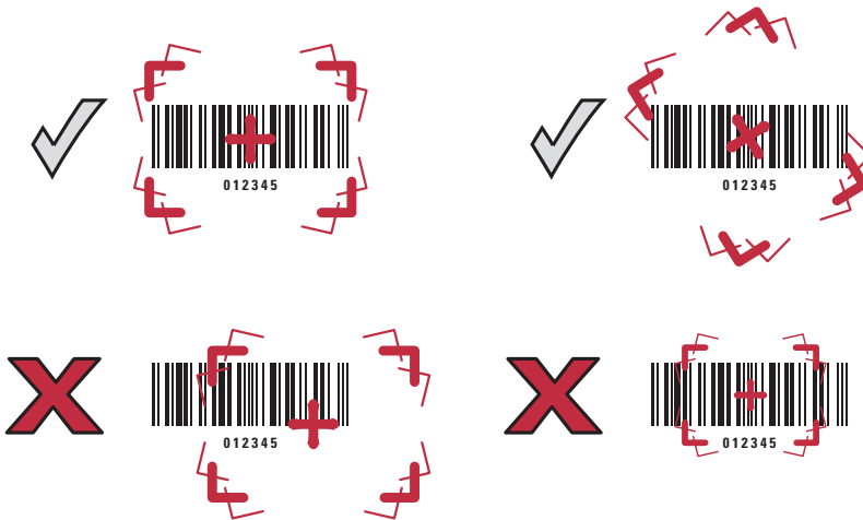
Figure 2-5 Acceptable and Incorrect Aiming - Standard Pattern
