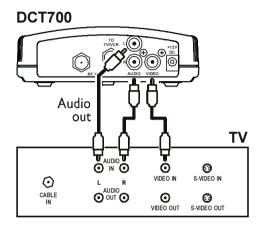
In these illustrations the baseband connectors on entertainment components are labeled R for right audio, L for left audio, and  $\vee$  or VIDEO.
