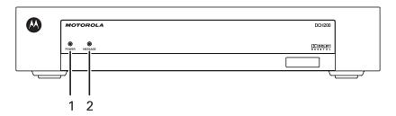
Power Indicator — Lit when the unit is powered ON, unlit when unit is OFF
