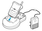
If desired, insert a spare battery (main or aux) into the desktop charger as shown.
