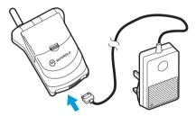
**4** Insert the power adapter plug into a 110V AC electrical outlet. A beep-tone sounds and the battery icon flashes when charging begins.
