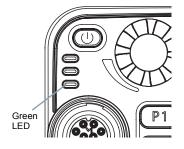
**NOTE:** The green LED lights up while the radio is transmitting and blinks rapidly when the radio is receiving a privacyenabled call.
