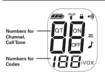
ON - On/Off for - Battery Meter OFF each feature (((j))) – 1 watt Channel
