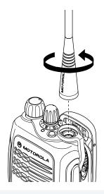
Turn the antenna counterclockwise to remove it.
