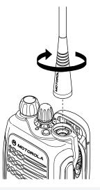
Turn the antenna clockwise to attach it.
