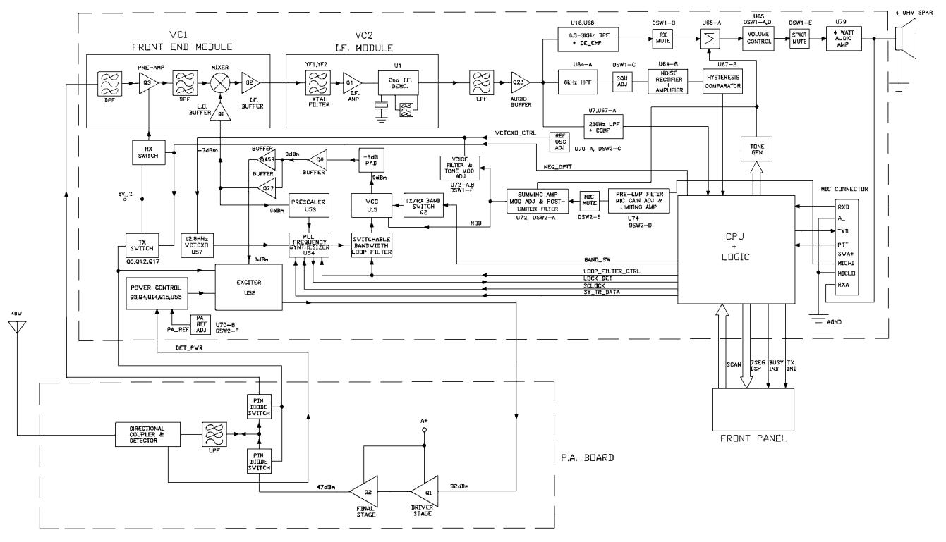
Figure 1 - MDS Conventional Radio Block Diagram
