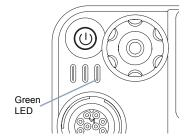
**NOTE:** The green LED lights up while the radio is transmitting and double blinks when the radio is receiving a privacyenabled call.
