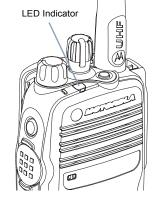
**Blinking yellow** – Radio is scanning for activity or receiving a Call Alert.
