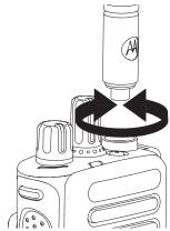
To remove the antenna, turn the antenna counterclockwise.
