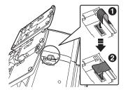
2. Attach the KX-NT305 to your unit with the screws.
