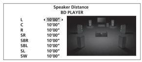
• The distance of all the speakers can be set to between 1 inch and 45 feet, in units of 1 inch.
