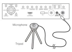
If you have a tripod, use it to place the microphone so that it's about ear level at your normal listening position. If you do not have a tripod, use some other object to install the microphone.  $^3$
