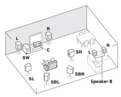
With these connections you can simultaneously enjoy 5.1-channel surround sound in the main zone with stereo playback of the same sound on the B speakers. The same connections also allow for 7.1-channel surround sound in the main zone when not using the B speakers.
