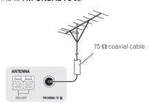
To improve AM reception, connect a 5 m to 6 m (16 ft. to 20 ft.) length of vinyl-coated wire to the  $\mathbf{AM}$  LOOP terminals without disconnecting the supplied AM loop antenna. For the best possible reception, suspend horizontally outdoors.
