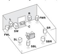
This plan replaces the left and right front height speakers shown in [A] with the left and right front wide speakers (FWL/FWR).<sup>1</sup>
