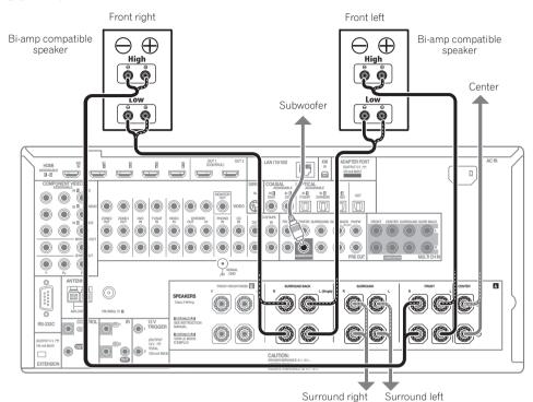
Bi-amping is when you connect the high frequency driver and low frequency driver of your speakers to different amplifiers for better crossover performance. Your speakers must be bi-ampable to do this (having separate terminals for high and low) and the sound improvement will depend on the kind of speakers you're using.
