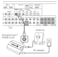
You will also need to connect the antenna and AC adapter to the SiriusConnect™ tuner.
