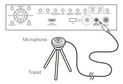
If you have a tripod, use it to place the microphone so that it's about ear level at your normal listening position. If you do not have a tripod, use some other object to install the microphone.<sup>1</sup>
