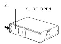
Insert the magazine firmly (which has been taken out of the unit) with the mark visible on the top side.
