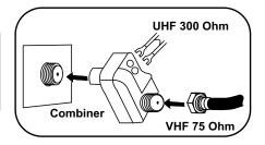
Connect the 75 Ohm cable from combination VHF/UHF antenna to the antenna jack.
