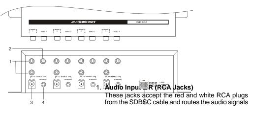
to the SDB (Signal Distribution Box) from the source component (Example VCP, DVD etc.). Use the SDBSC cable.
