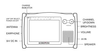
Charge indicator:Illumlinates when battreries are charging UHF/VHR Select/Power On/Off:Turns power on and off;Selects UHF/VHF TV band
