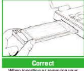
When inserting or removing your PCS Connection Card, grip the card by both of its sides.
