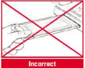
Do not handle or remove the PCS Connection Card by pulling on the antenna.
