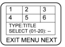
To remove the digest feature, use the direction buttons to select EXIT on the screen and press ENTER to confirm.
