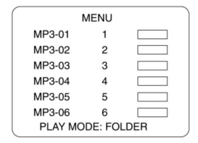
2.Press direction key ▼ to select song folder. Press ► (PLAY) to confirm selection. Example: Select MP3-02, the TV screen displays.
