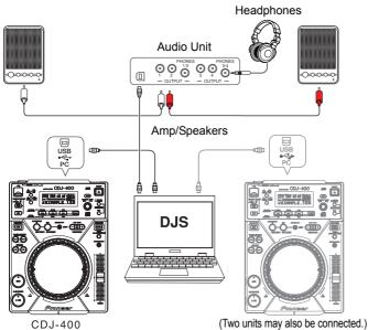
•Configuration when using an External DJ mixer (Example of Connections) The DJS player A and player B audio is output to each audio output of your computer. Your computer needs to have two or more audio output systems.
