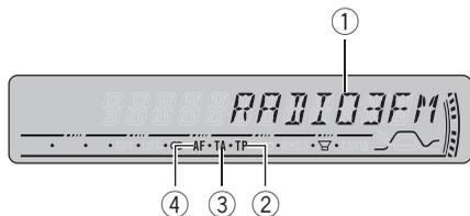
RDS (radio data system) is a system for providing information along with FM broadcasts. This inaudible information provides such features as program service name, program type, traffic announcement standby and automatic tuning, and is intended to aid radio listeners in finding and tuning in to a desired station.
