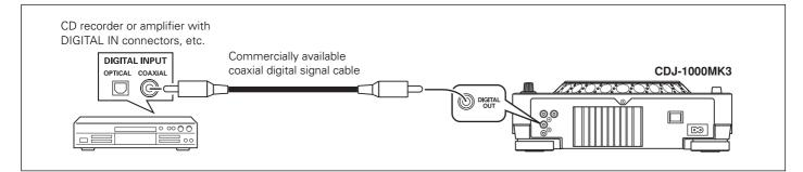
The DIGITAL OUT connectors produce audio data only (without subcodes; CD graphics are not supported).
