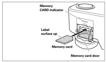
Open the memory card door, and insert the memory card, label side up and with the beveled edge toward the front. Insert the card slowly, holding it flat, and push it in until it stops. Shut the memory card door. The display will show [**SD CARD**] (for cards conforming to the SD memory card standard) or [**CDJ CARD**] (for cards formatted with the CDJ-1000 or CDJ-1000MK2), followed by the number of discs recorded on the card.
