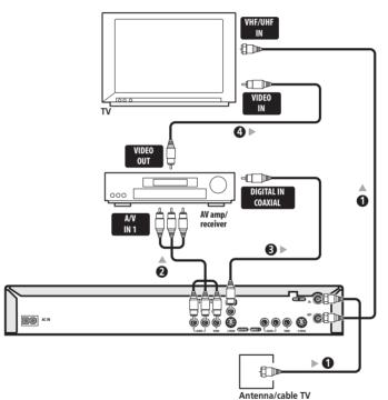
**1 Connect RF antenna cables as shown.** This enables you to watch and record TV channels.
