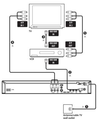
1 Connect your TV antenna/cable TV outlet to the VHF/UHF IN jack on this recorder.
