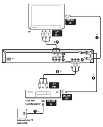
**1 Connect the RF antenna cables as shown.** This enables you to watch and record TV channels.
