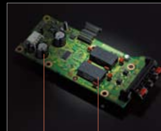
LOW IMPEDANCE CONDENSER LOW DISTORTION THIN CUSTOM COIL
