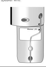
Turn the speakers towards the closest wall, lining the arrows up for optimal Front Surround. Turn each surround speaker so that the ▼ arrow at the base is lined up with the ▲ (FRONT SURROUND) arrow on the front speaker. This is only necessary when you are using the Front Surround mode (MODE ON). See the operating instructions for more on using Front Surround.
