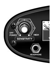
Sensitivity will be reduced slightly when using the Pioneer 101 in the Tone Discrimination mode. If you want optimal depth capability, operate in the All Metal mode by turning the Discriminate control completely counterclockwise; then turn the Sensitivity control clockwise to its highest clockwise position without chatter. If your Pioneer 101 chatters or beeps erratically, reduce the Sensitivity by turning the left knob counterclockwise.
