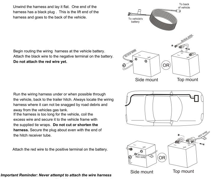
Important Reminder: Never attempt to attach the wire harness to a secondary power source, The lift requires direct connection to the battery.
