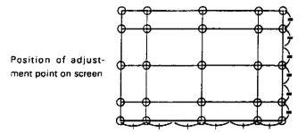
OIn point convergence adjustment, the 25 points set on the screen can be adjusted individually. In addition, the area of the four sides of the screen can be adjusted.
