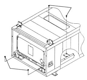
\*Drop the screw-lock fluid to screws so as not to loosen. (4 points)
