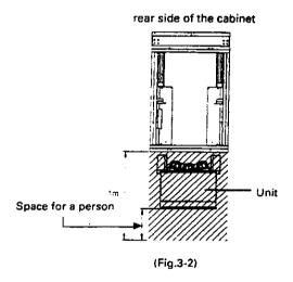
At installing locations where the projection unit has to be removed from the front, take note of how the unit is to be installed.(Refer to Chapter 3 4-(2)-3. Installation.)
