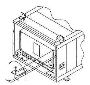
(12) Attach each rear panel (BMR1069, 1070, 1071, 1072) to the unit and the rear holders R and L using the screws (3  $\times$  8). Furthermore, to cover up the gap at the top of the projection unit, paste the hinder panel (BMR1075) over the top board and projection unit.
