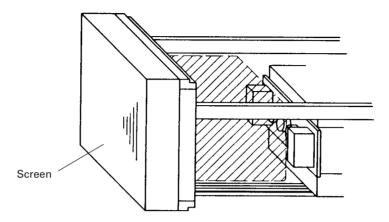
• When fixing the screen into the wall, space for placing your hand inside the wall at the top, bottom, right, and left will be required in addition to the above in order to attach and remove the screen.
