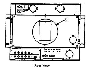
Remove the ⓐ panel of the rear panel shown in the left figure. When this panel is removed, there will be two printed circuit boards as shown in Fig. 4-1.
