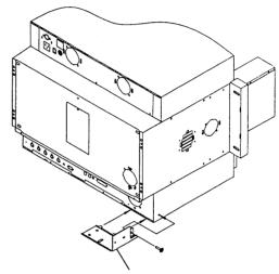
\*Drop the screw-lock fluid to screws so as not to loosen.(Right and left)
