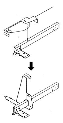
(4) Attach the parts assembled at steps (1) and (2) onto the multi-projection unit. Attach the attachments R and L to frajmes R and L. using the screw (M5  $\times$  15) as shown in the figure, and attach the attachments R and L to the rear of the projection unit using the screws (M5  $\times$  50). (2 screws  $\times$  2 locations).
