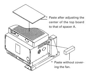
(7) Attach the attachments R and L to the unit through the top board of the unit using the screws (M6  $\times$  20) and then attach attachments R and L to the unit from the back using screws (M6  $\times$  20). (2 screws  $\times$  2 locations).
