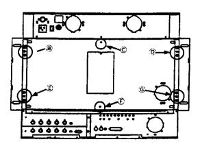
Remove the six screws 8 to 6 of the rear panel in the left figure.
