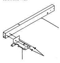
(2) Insert the claws of holders R and L (BNG1150, 1151) into the slits of frames R and L, rotate them as shown in the figure, and attach using the screws (M5  $\times$  15). (2 pieces  $\times$  2 locations).
