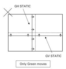
The center adjustment by H PHASE V PHASE adjusts the timing for displaying video signals and therefore current is not supplied to the deflection york.
