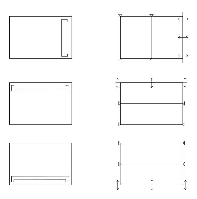
In adjustment step 111, observe the external part of the screen, adjust the 16 adjusting points there, taking note of linearity in the peripheral area such as joining with other screens, crosshatch, etc.
