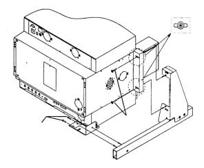
(5) Paste spacer A (BMR1073) to the top board of the multi-projection unit and spacers B (BMR1074) to the two sides at the position shown in the figure after peeling off the seal.
