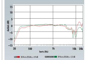
Mounted in a wall, both the Pioneer Elite S-IW571L and the Pioneer Elite S-IW871LR deliver smooth bass and midrange response but exhibit some anomalies in the tweeter range; both show a broad dip in the range from about 7 to 12 kHz. Off-axis response is fairly consistent out to 30° off-axis with both speakers. Both deliver fairly strong bass response between 40 and 80 Hz — average output at 10% distortion or lower is 88 dB for the S-IW571L and 93 dB for the S-IW871LR. — *B.B.*
