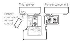
2 If the Pioneer component also has a CONTROL OUT jack, you can continue the chain in the same way for as many components as you have.
