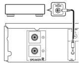
Connect the 12V TRIGGER jack of this receiver to the 12V trigger of another component.
