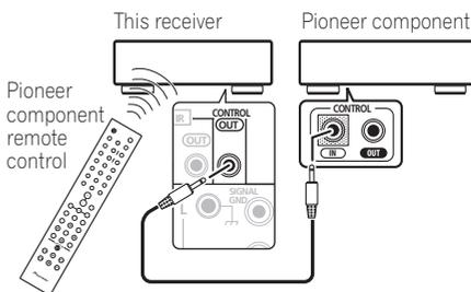
**2 If the Pioneer component also has a CONTROL OUT jack, you can continue the chain in the same way for as many components as you have.**
