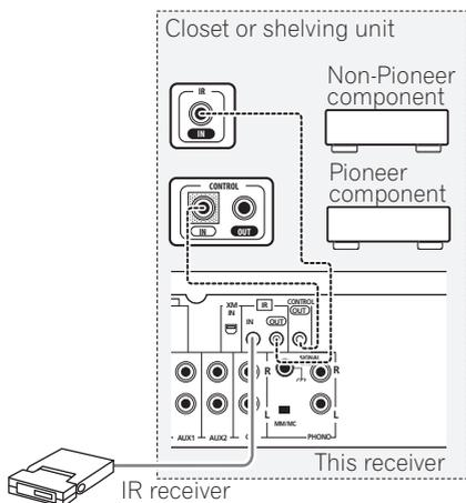
**2 Connect the IR IN jack of another component to the IR OUT jack on the rear of this receiver to link it to the IR receiver.**
