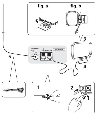
**1 Pull off the protective shields of both AM antenna wires.**
