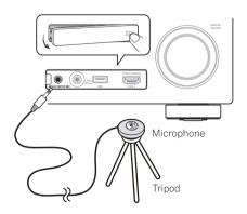
If you have a tripod, use it to place the microphone so that it's about ear level at your normal listening position. If you do not have a tripod, use some other object to install the microphone.<sup>1</sup>
