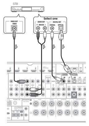
If your set-top box is equipped with an HDMI output terminal, we recommend connecting it to the receiver's HDMI IN terminal. When doing so, also connect the receiver and TV by HDMI (see Connecting using HDMI on page 24).
