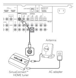
You will also need to connect the antenna and AC adapter to the SiriusConnect™ tuner.
