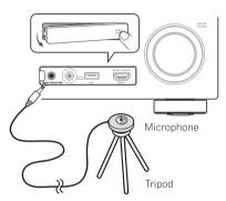
If you have a tripod, use it to place the microphone so that it's about ear level at your normal listening position. If you do not have a tripod, use some other object to install the microphone.<sup>3</sup>
