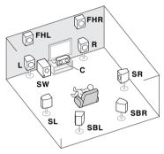
A 7.1 ch surround system connects the left and right front speakers (**L/R**), the center speaker (**C**), the left and right front height speakers (**FHL/FHR**), the left and right surround speakers (**SL/SR**), the left and right surround back speakers (**SBL/SBR**), and the subwoofer (**SW**).<sup>1</sup>
