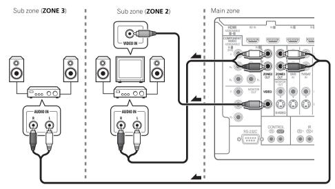
Different sources can be playing in three zones at the same time or, depending on your needs, the same source can also be used. The main and sub zones have independent power (the main zone power can be off while one (or both) of the sub zones is on) and the sub zones can be controlled by the remote or front panel controls. However, you may need to specify the volume settings in *ZONE Audio Setup* on page 89.
