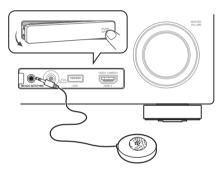
If you have a tripod, use it to place the microphone so that it's about ear level at your normal listening position. If you do not have a tripod, use some other object to install the microphone.<sup>1</sup>
