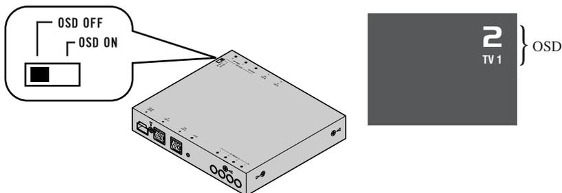
Set the OSD (On Screen Display) switch on the right side of this product to the appropriate position with a pen tip or other pointed instrument, for the component you are combining it with.
