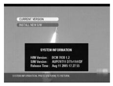
Under the CURRENT VERSION submenu, the ID number of installed hardware and software versions of the tuner are displayed.
