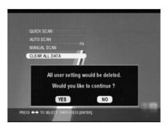
This option allows you to reset the tuner to its factory settings, losing all channels and setup changes you have made. Select CLEAR ALL DATA to reset the tuner.
