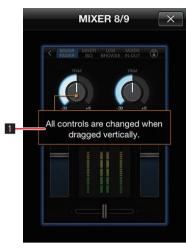
For all of the controls, the level can be adjusted by dragging vertically.
