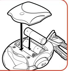
2. Insert 2 new "AA" alkaline batteries
