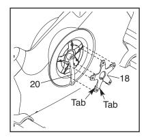
Cover (18). Carefully work the left Disc Cover over the Left Crank Arm (20) and remove the left Disc Cover.
