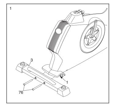
2. Attach the Front Stabilizer (2) to the Frame (1) with two M10 x 95mm Patch Screws (76).
