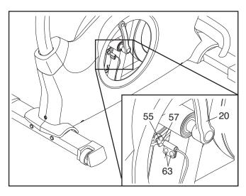
Next, rotate the Left Crank Arm (20) until a Magnet (55) is aligned with the Reed Switch (57). Slide the Reed Switch slightly toward or away from the Magnet. Then, retighten the M4 x 12.7mm Flange Screws (63).
