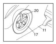
left Pedal Disc upward and remove it from the Left Crank Arm (20).
