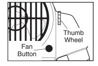
the fan, press the fan button a third time. Note: If the fan is turned on but the pedals are not moved for thirty seconds, the fan will automatically turn off to conserve the batteries.
