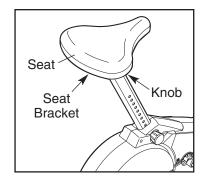
turn the indicated knob counterclockwise two or three turns to loosen it (if the knob is not loosened enough, it may scratch the seat bracket). Next, pull the knob, slide the seat to the desired position, and then release the knob. Move the seat bracket forward and backward slightly until the pin on the knob snaps into one of the holes in the seat bracket. Then, turn the knob clockwise until it is tight.
