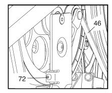
shields; there are three sizes of screws in the shields—note which size of screw you remove from each hole. Then, gently pry the shields away from the frame.
