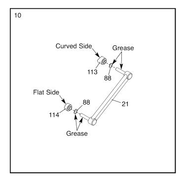
11. At the same time, insert a Pedal Arm Axle (21) into the Right Upper Body Leg (31) and into the right Pedal Arm (14); make sure that the Upper Body Leg Spacer (113) and the Pedal Leg Spacer (114) are in the indicated locations.
