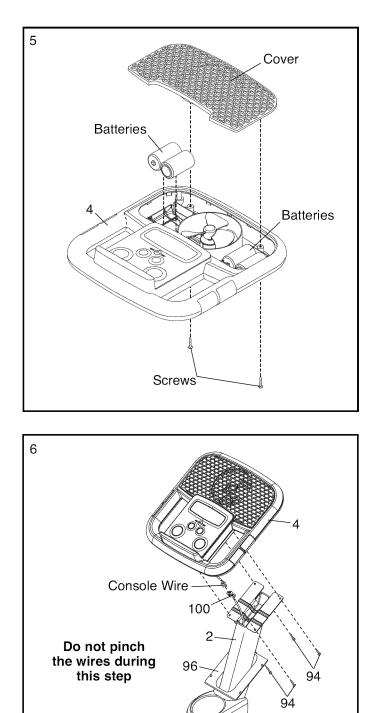
Slide the Console Cover (96) (see the drawing in step 6) upward to the Console (4). Attach the Console Cover with four M4 x 16mm Screws (84).
