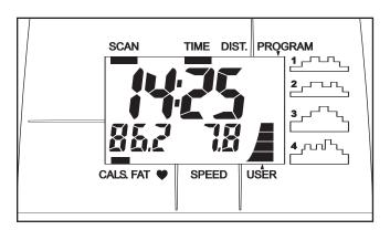
Time—This mode displays the elapsed time (or the time remaining in a pace program). Note: If you stop pedaling, the time will begin to flash.
