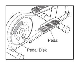
other pedal. Push the pedals until they begin to move with a continuous motion. Note: The pedal disks can turn in either direction. It is recommended that you turn the pedal disks in the direction shown above; however, for variety, you can turn the pedal disks in the opposite direction.
