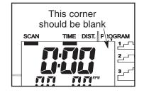
mode by pressing the Program button repeatedly until the upper right corner of the display is blank.
