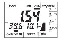
play will then show only the elapsed time, and the lower left section of the display will show only the number of calories you have burned. Press the Mode button again. The upper section of the display will then show only the distance pedaled, and the lower left section of the display will show only the number of fat calories you have burned. To select the scan mode again, press the Mode button repeatedly until a mode bar appears below the word SCAN.
