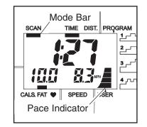
nately show the elapsed time and the distance that you have pedaled; the lower left section of the display will alternately show the number of calories you have burned and the number of fat calories you have burned; and the lower right section will show your pedaling speed.
