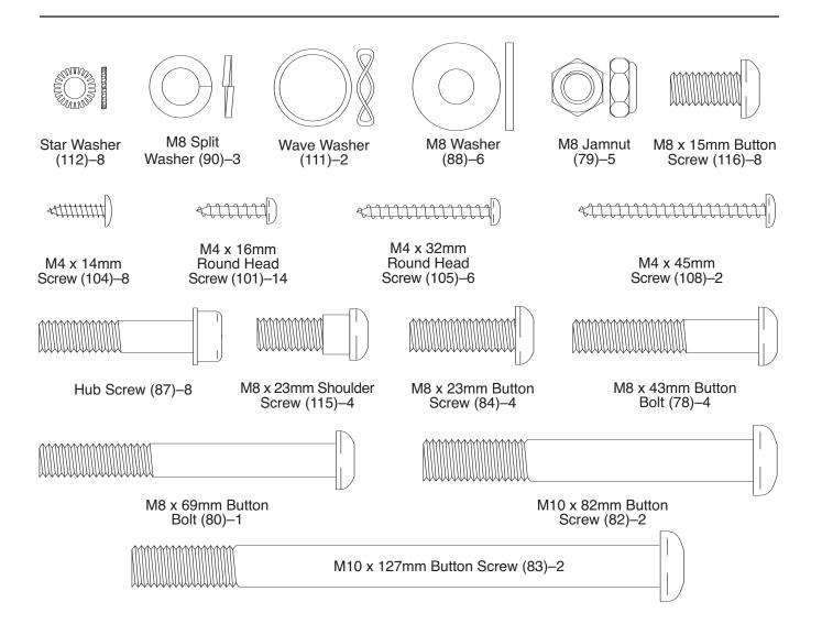
While another person lifts the Base (1), attach the Front Stabilizer (6) to the Base with two M10 x 82mm Button Screws (82).
