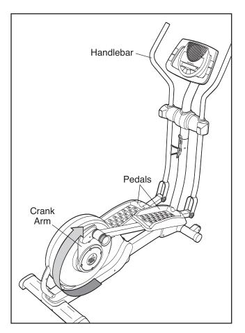
To dismount the elliptical exerciser, wait until the pedals come to a complete stop. **Note: The elliptical exerciser does not have a free wheel; the pedals will continue to move until the flywheel stops.** When the pedals are stationary, step off the highest pedal first. Then, step off the lowest pedal.
