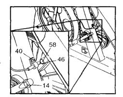
remove, the indicated M4 x 16mm Screw (40). Slide the Reed Switch slightly closer to or away from the Magnet. Retighten the Screw. Turn the Crank Arm for a moment. Repeat until the console displays correct feedback. When the Reed Switch is correctly adjusted, reattach the left side shield, the side shield cover, and the left pedal.
