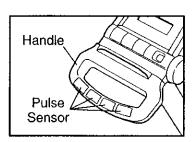
To use the pulse sensor, hold the handle on the console, with your right palm covering the two right contacts and your left palm covering the two left contacts. Avoid moving your hands. When your pulse is detected, the heart-shaped indicator in the display will flash each time your heart beats and two dashes (--) will appear. After a moment, your heart rate will be shown. For the most accurate heart rate reading, continue to hold the handgrips for about 15 seconds.
