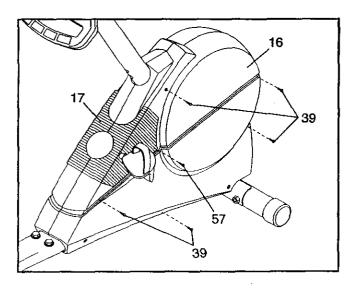
Using an adjustable wrench, turn the Left Pedal (20) clockwise and remove it. Next, remove the two M4 x 16mm Screws (40) from the Left Side Shield (15) and the M4 x 12mm Screw (57) from the Side Shield Cover (17). Lift off the Side Shield Cover and the Left Side Shield.
