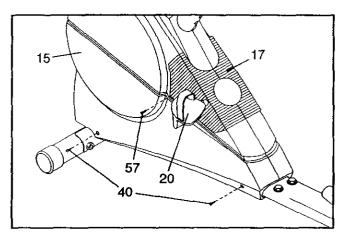
Next, locate the Reed Switch (46). Turn the left arm of the Crank (14) until the Magnet (58) is aligned with the Reed Switch. Loosen, but do not
