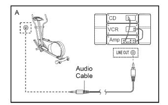
B. Plug one end of a 1/8" to RCA stereo audio cable (available at electronics stores) into the jack beneath the console. Plug the other end of the cable into an RCA Y-adapter (available at electronics stores). Next, remove the wire that is currently plugged into the LINE OUT jack on your stereo and plug the wire into the unused side of the Y-adapter. Plug the Yadapter into the LINE OUT jack on your stereo.
