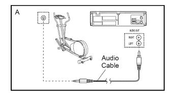
B. Plug one end of a 1/8" to RCA stereo audio cable (available at electronics stores) into the jack beneath the console. Plug the other end of the cable into an RCA Y-adapter (available at electronics stores). Next, remove the wire that is currently plugged into the AUDIO OUT jack on your VCR and plug the wire into the unused side of the Yadapter. Plug the Y-adapter into the AUDIO OUT jack on your VCR.
